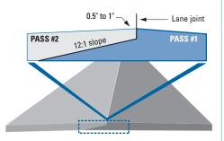
The key elements to a successful wedge joint are creating a <sup>1</sup>/<sub>2</sub>" to 1" notch at the inner edge of the wedge, with a 12:1 taper ratio, and compacting the wedge with a steel roller. A tack coat on the wedge before the second lane is placed produces good adhesion.
