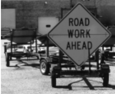
Sign trailers like these don't meet the new standards. New trailers should not be acquired, but existing ones may continue in use for a few years.
