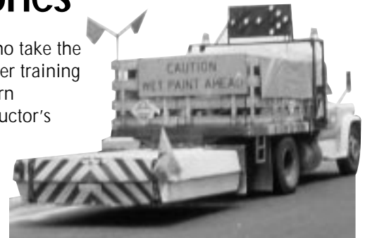
Some agencies are adding crash attenuators behind trucks for worker safety.
