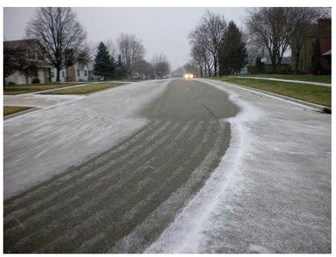
A test street in De Pere during a snow event illustrates the impact of an anti-icing operation. Treated pavement resists initial snow and ice accumulation prior to plowing.
