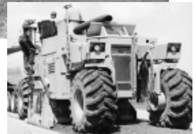
Reclaiming uses old asphalt pavement to strengthen the road.
