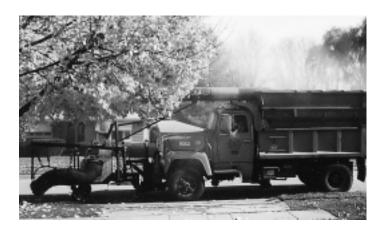
The first leaf collector was specially modified for Ripon by American Roads of Ohio. A pull-behind leaf loader was set on a custom-wheeled frame and had hydraulic cylinders installed to move the hose. It cost about \$20,000 in 1987. In 1992, using city forces, they modified a second one using an older pull-behind leaf vac. The cost was just under \$8000.
