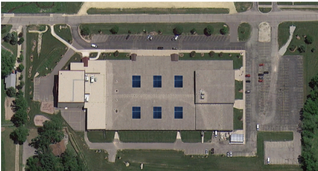
Figure 11: The general rooftop arrangement for a 100 kW photovoltaic system. The system contains 6 rows of 3 x 20 module panels, which would be directed south at latitude tilt.
