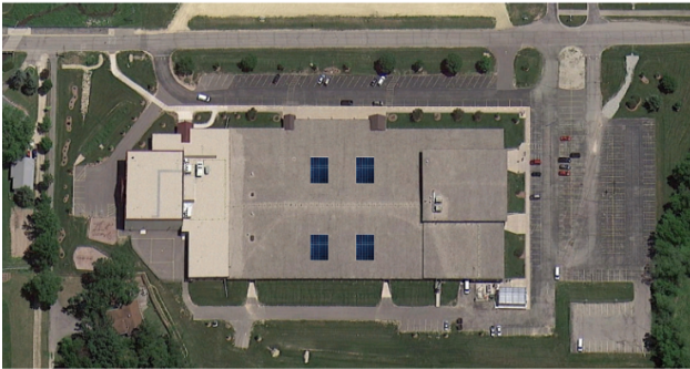
Figure 12: The general rooftop arrangement for a 10 kW photovoltaic system. The system contains 4 rows of 2 x 5 module panels, which would be directed south at latitude tilt.
