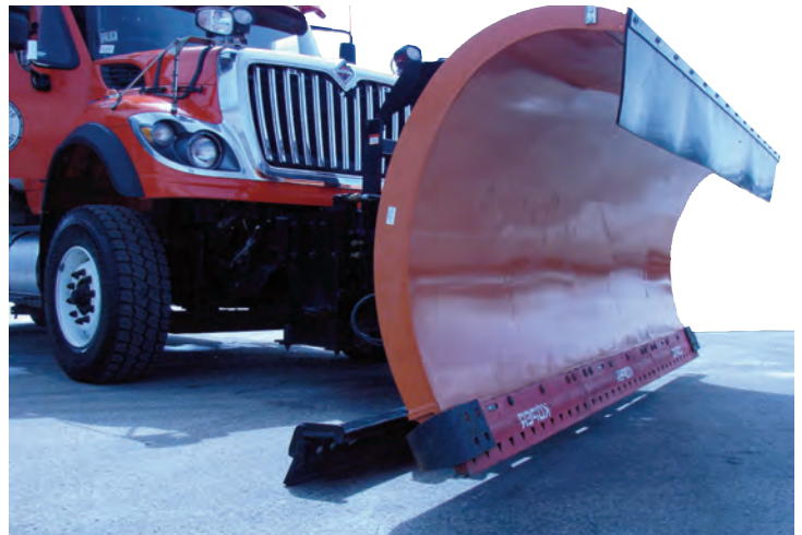
McHenry County plow operators use this two-blade plow configuration to remove snow and slush on their northern Illinois roads. The county is one of the first in the U.S. to experiment with multi-edge plows.
