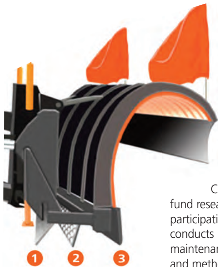
Drawing above shows a multi-edge, 3-blade plow configuration with 1) a squeegee blade at the back to clear slush, 2) a scarifying blade in the middle to break up snow pack and 3) the main snow blade in front.
