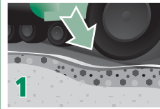
1 Vehicle weight causes pavement to bend slightly.
