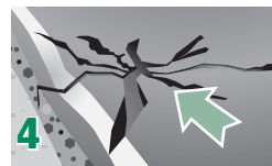
4 Vehicle traffic eventually compresses the weakened pavement over the cavity and the crack becomes a pothole.
