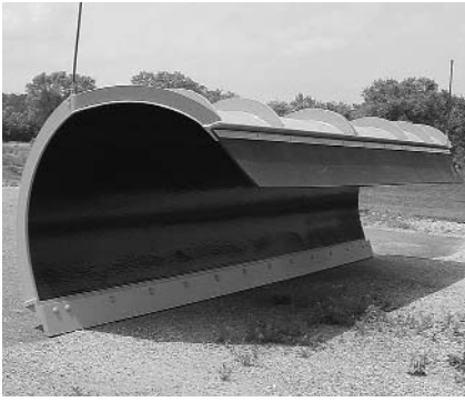
Plastic reduces drag on the plow moldboard.
