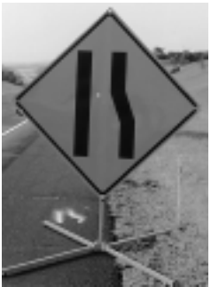
This X-footprint support and roll-up sign are crashworthy under FHWA's new standards.
