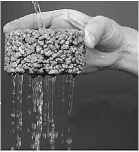
Water draining through pervious concrete.
