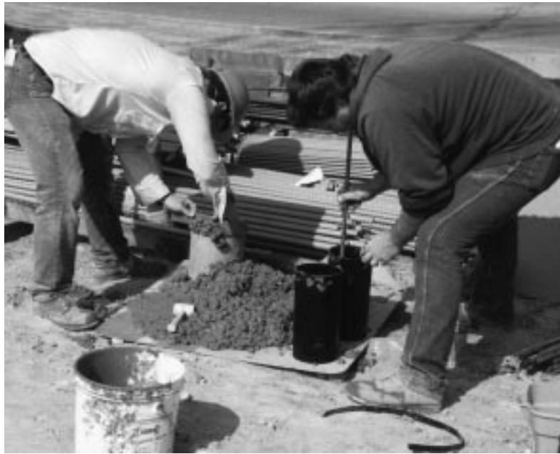
To ensure accurate test samples, fill, rod, and surface cylinders properly.
