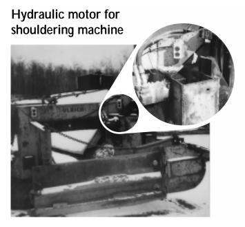
When their shouldering machine's gearbox wore out, Sawyer County, Wisconsin, Shop Foreman Jay Sands decided to replace it with a hydraulic motor. The gear system made it difficult to run the shouldering belt slowly at low speeds. The hydraulic replacement has smoothed out the problems. The system includes a hydraulic motor and pump to run the belt. Cost of parts to convert to the hydraulic system was \$2835 and installation took about 75 hours.
