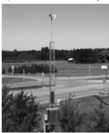
maintenance. Wisconsin now has a network of pavement sensors and weather stations on Interstates and other major divided highways. The stations continuously report weather and pavement data via personal computer to all County Highway offices, WisDOT District offices, and other municipalities.
