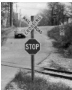
STOP signs should not be mounted on the railroad crossing crossbucks.
