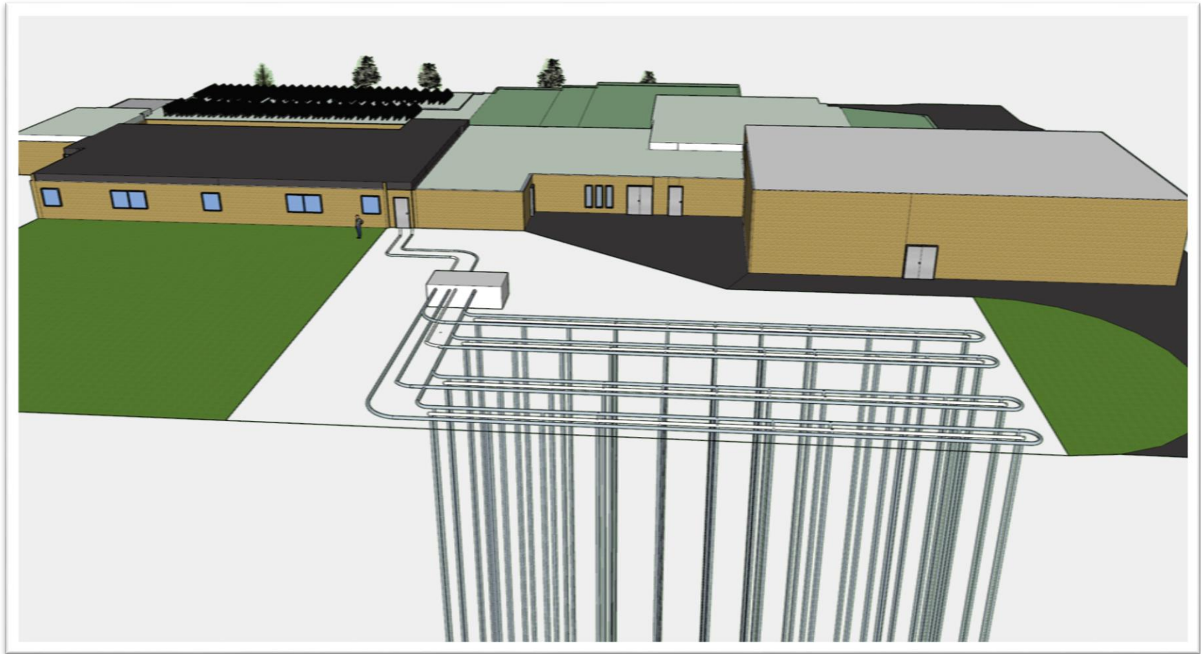
Figure 2. Rendering of the 44-vertical borehole geothermal energy system, looking east.
