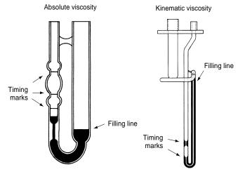
Figure 5. Viscometers for asphalt cement
