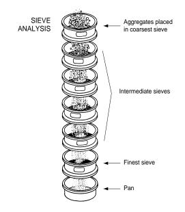
Figure 4. Determining size and gradation of aggregates
