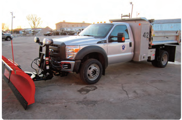
The Oshkosh Parks Department attaches a plow blade to this CNG-powered one-ton truck to clear parking lots of snow in winter.
