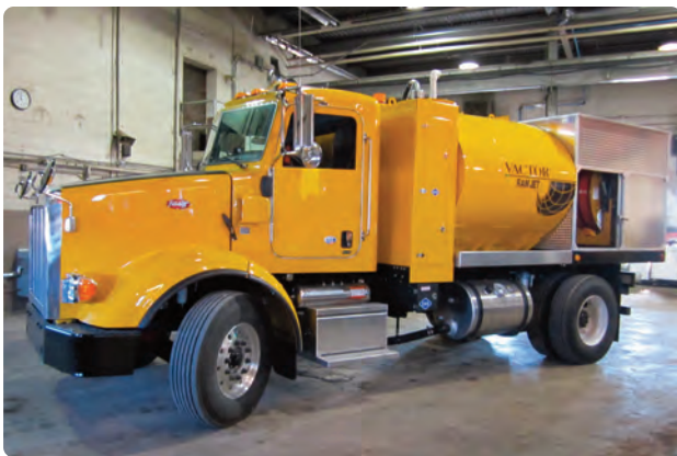
City of Oshkosh camera truck, used in sewer operations, has separate CNG engines to power it and run a compressor.
