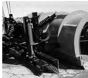
A multi-blade system from Monroe Truck Equipment features a carbide blade backed by an ice blade and a rubber blade.
