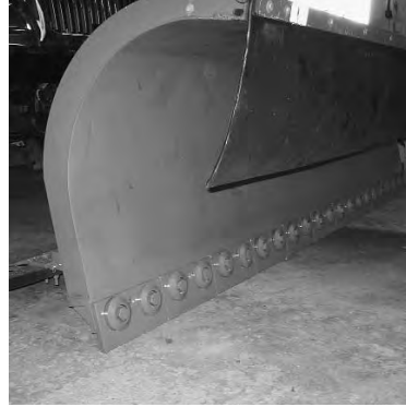
IADOT tested the Polar Flex rubber carbide blade by Valley Blades LEFT last year and an in-house prototype RIGHT with one-foot carbide sections and rubber.
