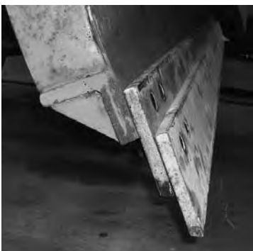
Stacked standard carbide blades on an IADOT plow.
