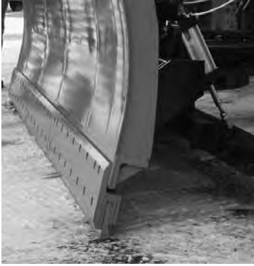
IADOT tested the Polar Flex rubber carbide blade by Valley Blades LEFT last year and an in-house prototype RIGHT with one-foot carbide sections and rubber.
