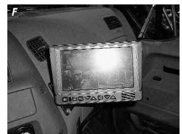
(photo F) inside the cab has a four-way split screen that allows the operator to check regularly for visual cues in each position. ■
