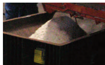
Participants learned that a tarp and bucket TOP are effective stand-ins for a hopper and electronic scales BOTTOM in calibrating salt and sand spreaders.
