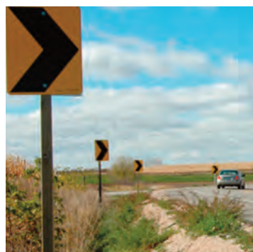
Installing chevrons on curves is an improvement that qualifies for HSIP funds.
