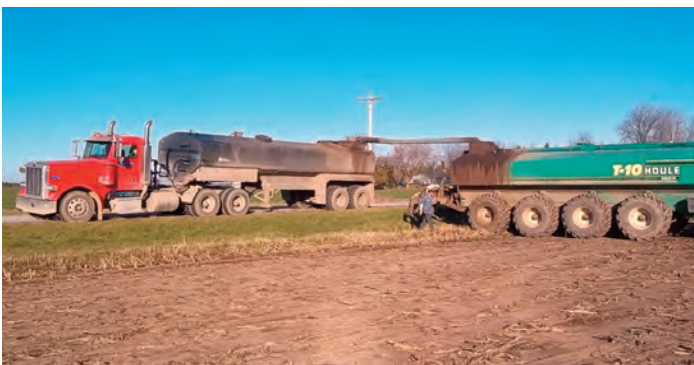
Eisentraut AG sometimes moves materials from farm to field by transferring loads from a tanker on the road to spreaders in the field, avoiding the need to drive a heavier vehicle on town roads.
