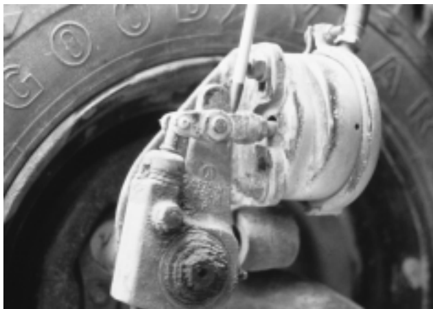
Inspect brake slack adjusters daily. Truck brakes are often out of adjustment.
