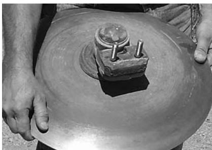
UPPER LEFT "Gravel saver" disk mounted on the moldboard. BOTTOM LEFT The disk has a simple mount. BOTTOM RIGHT Disk keeps gravel from flowing around the toe of the moldboard.
