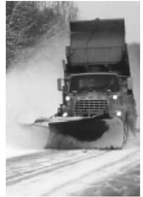
Adding wings substantially cuts residential plowing times.
