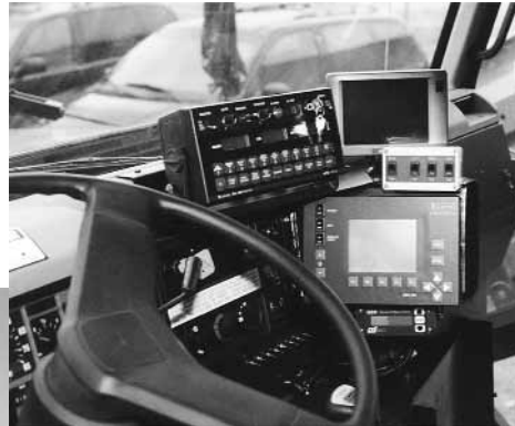
A small tv monitor in the cab shows salt-spreading and traffic conditions behind the truck as seen by rear mounted cameras.
