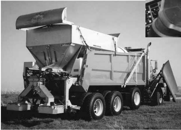
Combining liquid anti-icing tanks with conventional spreaders is efficient and saves salt.
