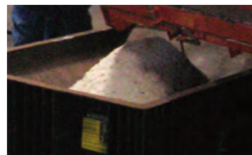
Participants learned that a tarp and bucket TOP are effective stand-ins for a hopper and electronic scales BOTTOM in calibrating salt and sand spreaders.
