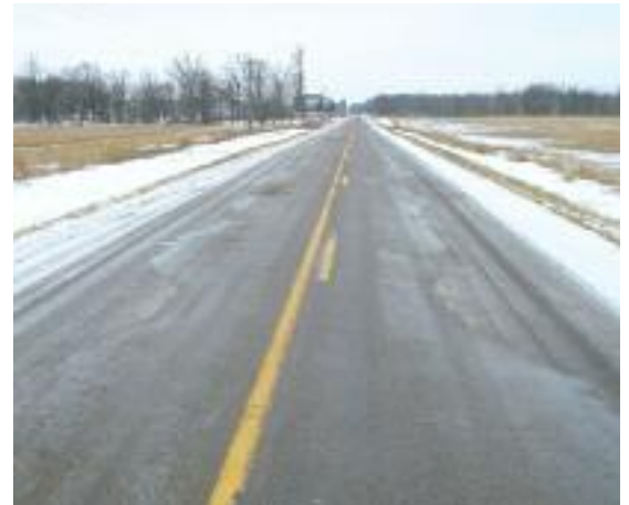
Photos taken during the pilot show the results on a county road, left, treated with salt sand only (600 lbs per lane mile) and one with salt sand (400 lbs per lane mile) plus the recycled salt brine, right. Fifteen minutes after application, the salt brine road was 50 percent clearer than the one without the de-icer.
