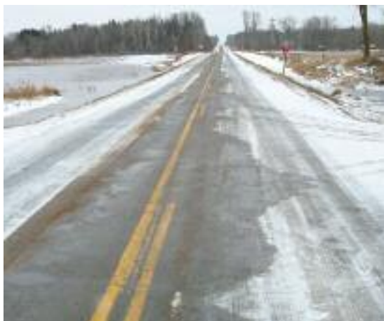
Photos taken during the pilot show the results on a county road, left, treated with salt sand only (600 lbs per lane mile) and one with salt sand (400 lbs per lane mile) plus the recycled salt brine, right. Fifteen minutes after application, the salt brine road was 50 percent clearer than the one without the de-icer.
