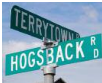
Replace all-uppercase lettering on post-mounted street name signs, like this one, with a combination of uppercase and lowercase letters by January 2012.
