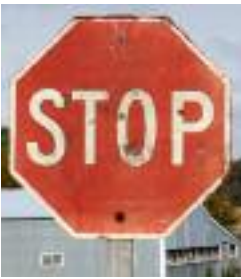
Faded and with little or no retroreflectivity, this STOP sign is past due for replacement.
