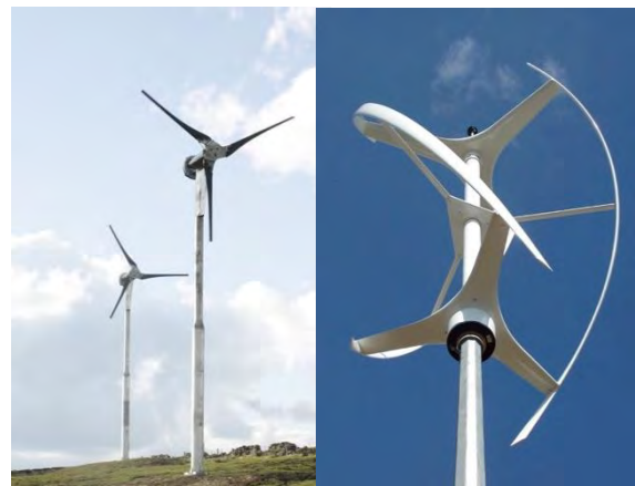
FIGURE 1: HORIZONTAL AXIS WIND TURBINE (LEFT). VERTICAL AXIS WIND TURBINE (RIGHT).
