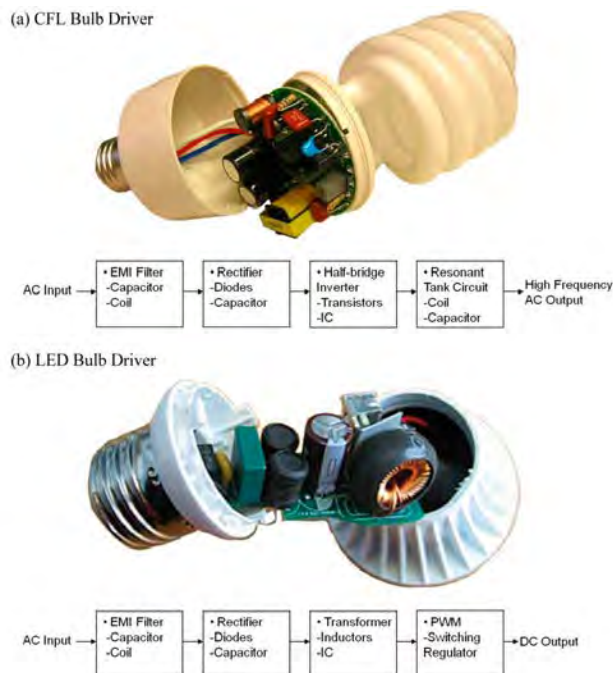
Figure A7: Internal components of CFL (a) and LED (b) lightbulbs.
