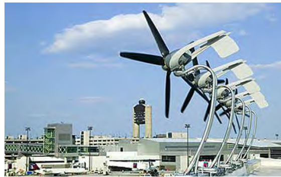
FIGURE 3: SMALL SCALE HORIZONTAL AXIS WIND TURBINES LOCATED ON ROOFTOP OF A BUILDING (McDERMOTT, 2009).
