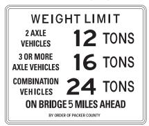
Bridge weight restriction signs must follow instructions from WisDOT. These signs must include the gross weight and maximum limits for axle loads. Signs should be posted at the bridge and also far enough in advance that trucks can detour around the limited structure.
