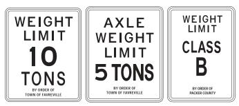
Temporary weight limits such as spring load restrictions should also be on standard signs that are reflectorized and that meet the standards of the *MUTCD*. Hand painted and faded signs are not appropriate.
