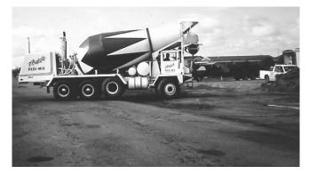
Another factor is the amount of weight and number of tires on each axle. Damage increases rapidly with higher axle loads and actually worsens at a faster rate than the load increases. A nine-ton axle load, for example, causes about ten times more damage than a five-ton axle load. Distributing a vehicle's weight and its payload over more axles and tires makes the load lighter at each point of contact, reducing damage to the road.
