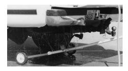
using 1-inch PVC pipe, lawn mower wheels, and pressure nozzles. The wash is 105 inches long and 48 inches wide. It has two cross tubes with 15 pressure nozzles. The nozzles are adjusted to spray in various directions. The water pressure is generated by a gas-powered water pump.
