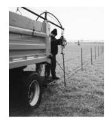
bolted to the back frame of the truck lets two people operate the pounder with power from a portable air compressor in the truck.
