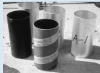
Cylinder types: metal, plastic and paper.
