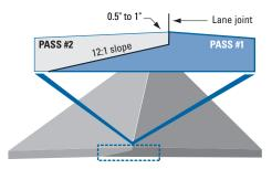
The key elements to a successful wedge joint are creating a 1/2" to 1" notch at the inner edge of the wedge, with a 12:1 taper ratio, and compacting the wedge with a steel roller. A tack coat on the wedge before the second lane is placed produces good adhesion.
