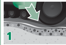
1 Vehicle weight causes pavement to bend slightly.
