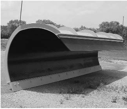
Plastic reduces drag on the plow moldboard.
