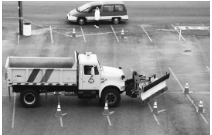
Diminishing clearance maneuvers test how well the driver knows the blade clearances, a skill that helps prevent sideswipe crashes (below).
