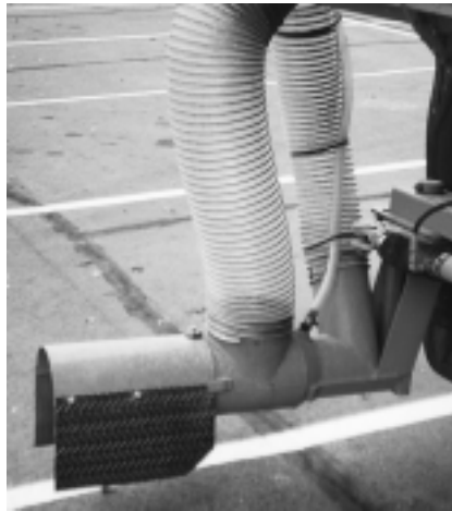
Zero velocity application means more deicing material stays on the road than with a conventional spinner.
