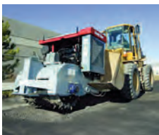
Asphalt Zipper reclaimer attached to wheel loader.
