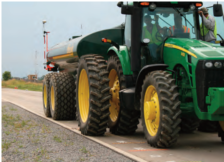
The study measured different load levels over five days of testing on the flexible pavement sections in each of the spring and fall test periods. Experienced drivers drove tankers like this one, empty and with loads at 25, 50, 80 and 100 percent capacity.
