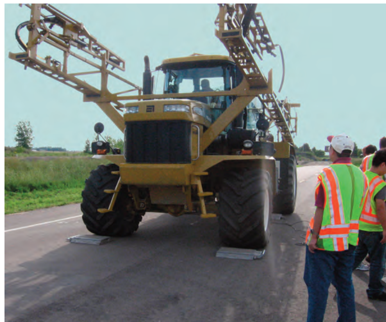
The road researchers used portable scales to measure the weight of all study vehicles at the start of each test period, as with this double-axle applicator. It was one of two applicators tested that produced some of the highest stresses and strains recorded.
