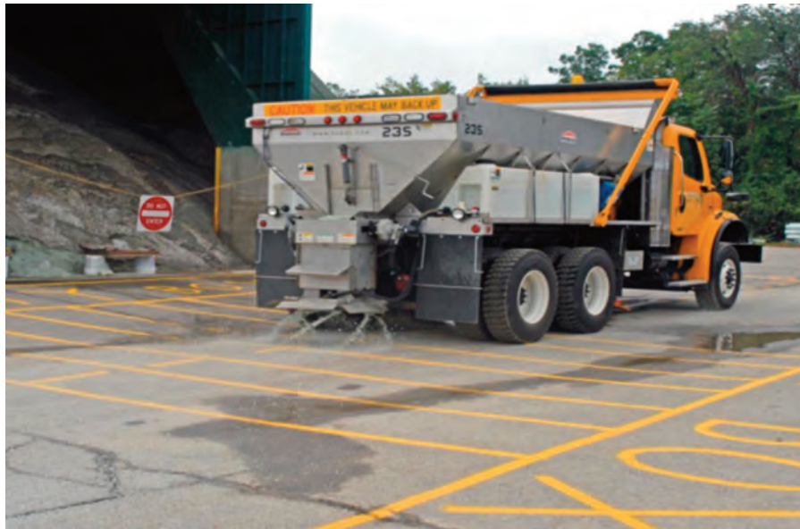
Street and highway departments can use a materials application grid like this to observe the scatter of salt delivered at various spreader and spinner speeds.
