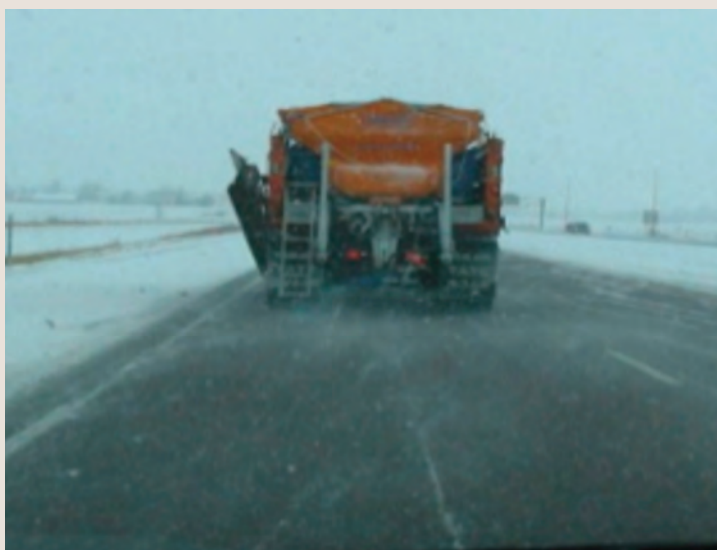
More salt stays in the target zone at lower speeds. A spreader traveling at 35 mph can send 50 percent or more into the ditch. At 25 mph, salt loss is down to about 22 percent.
