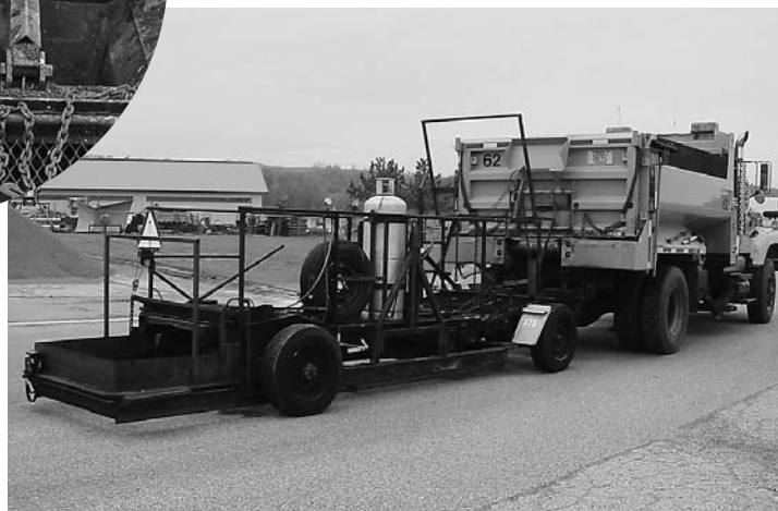
Rut-filling sled rides tandem behind truck carrying hot asphalt mix. INSET: Hopper mounted between feeds mix to slider.
