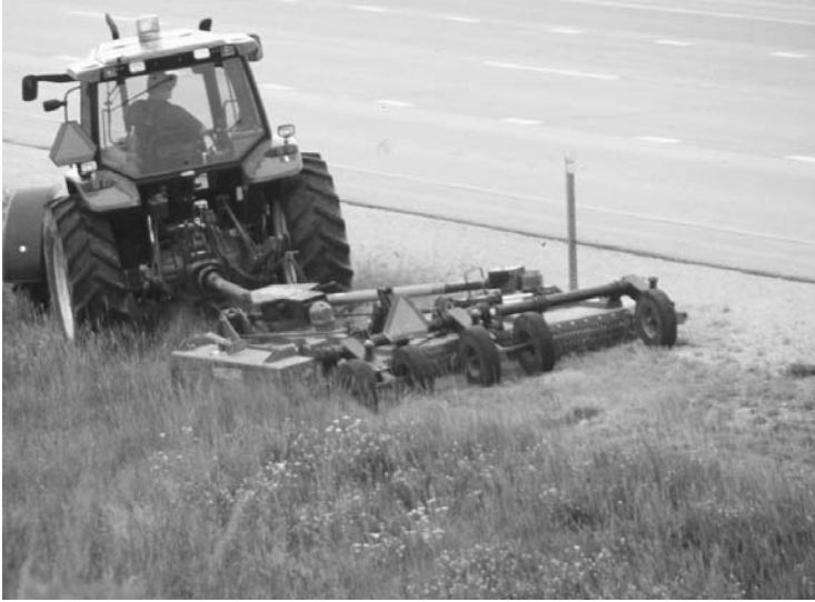
Mowing to prevent fires and keep a clear zone for pull-offs is a big part of every local roads management program.
