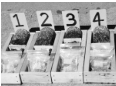
Cores show different results from the four reclaiming methods.
