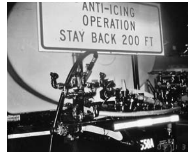
Flink anti-icing system mounted on back of tanker.
