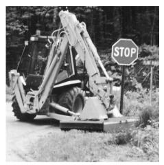
"We can use it all year round as a loader-tractor-backhoe and mower tractor," says Sleeter. "We can even use it for heavy brushing by planting the down-riggers and extending the stick."
