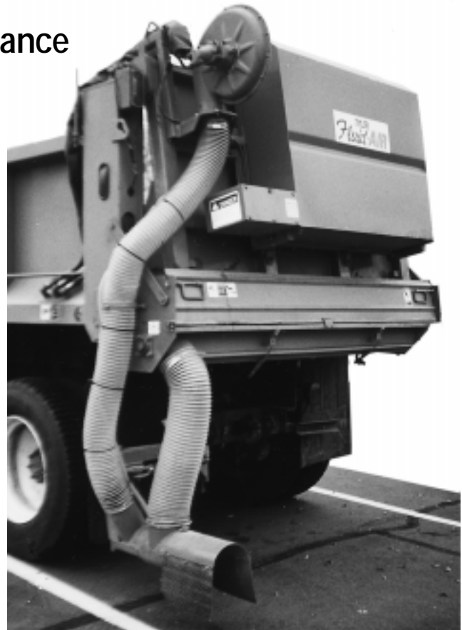
This truck is fitted with new snow and ice fighting equipment: a zero-velocity spreader and pre-wetting system.
